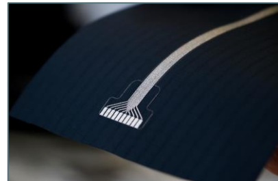
Printed OTech Jet silver electrode on textile
