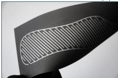
Printed OTech Jet silver electrode on paper
